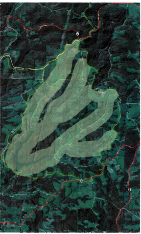
Barnesville's Slope Creek Reservoir. The reservoir's watershed is illustrated with the yellow line. The shaded area represents the source water protection area.
